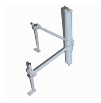
The picture above shows an assembled spike mount. There is one more leg that should may be attached for better stability, but for alignment purposes, only two legs and the center spike should be touching the ground. The 3<sup>rd</sup> leg is lowered after the alignment.
